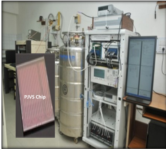
Established PJVS system at CSIR-NPL India for quantum DC voltage metrology
