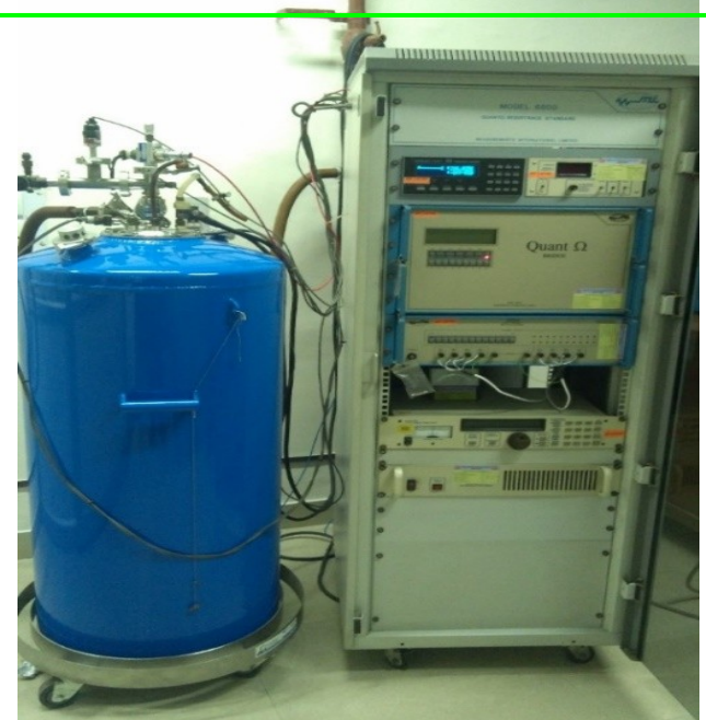
Primary Resistance Standard at CSIR-NPL provides resistance traceability to Temperature, DC and LF/HF standard at CSIR-NPL which disseminates to respective industries.
